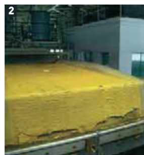
2 Uranium ore being processed into yellow cake at the mill at Jaduguda in Jharkhand.
