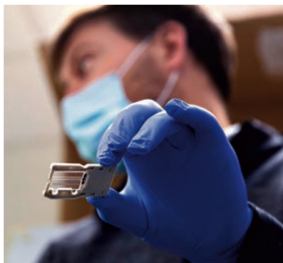
A FLOW CELL used for sequencing the coronavirus at a lab in Seattle, April 15. Analysing a virus' genetic code lets researchers track its mutations.
